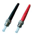
At D-Link, we adopt high precision equipments in fiber connectors product line providing the highest levels of reliability and performance. Each connector has a 2.5mm ceramic ferrule which is housed in a nickel plated brass housing. Available in both Single and Multi mode, connectors come with a 900µm and 3mm strain relief boot. Good for use with pigtail and buffered fiber cables.
